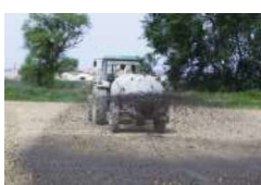
Tradicional broadcasting application of pig slurry.
